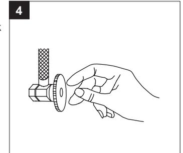
5. Remove aerator (5.1) from the spout. Turn on the faucet (A) and run the water for at least 30 seconds to flush out water lines. Turn off the faucet (A) and replace aerator (5.1).
