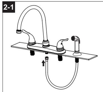
3. Connect the Water Supply Lines using a flexible braided supply line (3.1) (not included), connect the end with 1/2 in. female IPS to the tailpiece (3.2) of the faucet. Hand tighten. Do not overtighten. Install the other end of the supply line (3.1) to the shut-off valve or supply tube.
