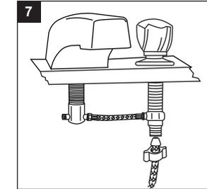
8. Turn water supply or shut-off valve back on and check for leaks. If leaks occur, tighten nuts slightly.
