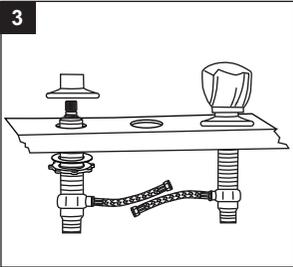
4. Install handles and secure with handle screws. Snap in hot and cold buttons.
