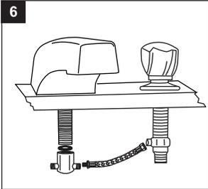
7. Attach water supply lines to end valves.
