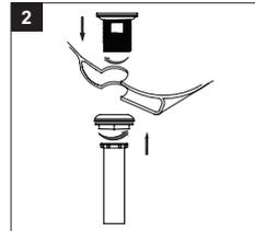
3. From underside of the sink, slide the rubber washer with beveled side down toward sink onto the drain body. Secure the drain body to the sink using nut. **DO NOT OVERTIGHTEN.**
